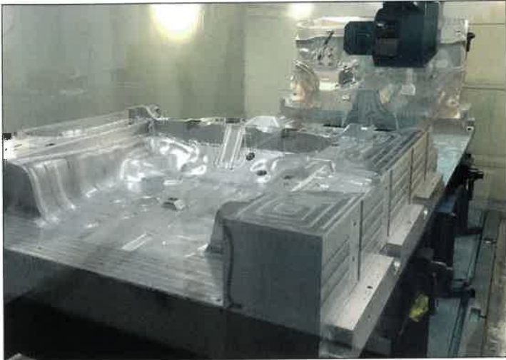
Fig. 1 — Subtractive machining of a geometrically complex aluminum-gauging tool for checking automobile polymeric shapes.
