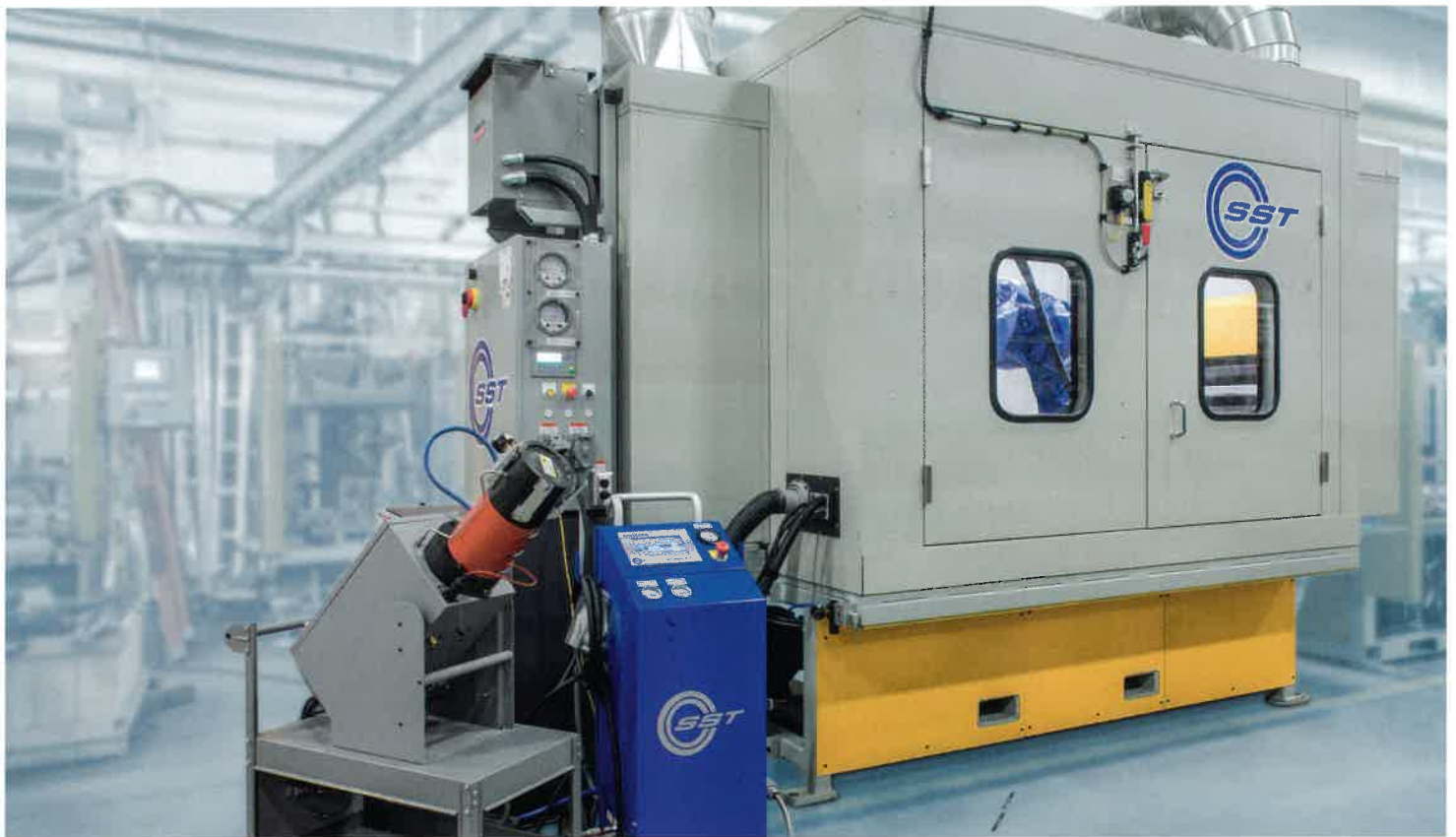
A commercial SST cold spray system. (Photo courtesy of CenterLine (Windsor) Ltd.)
